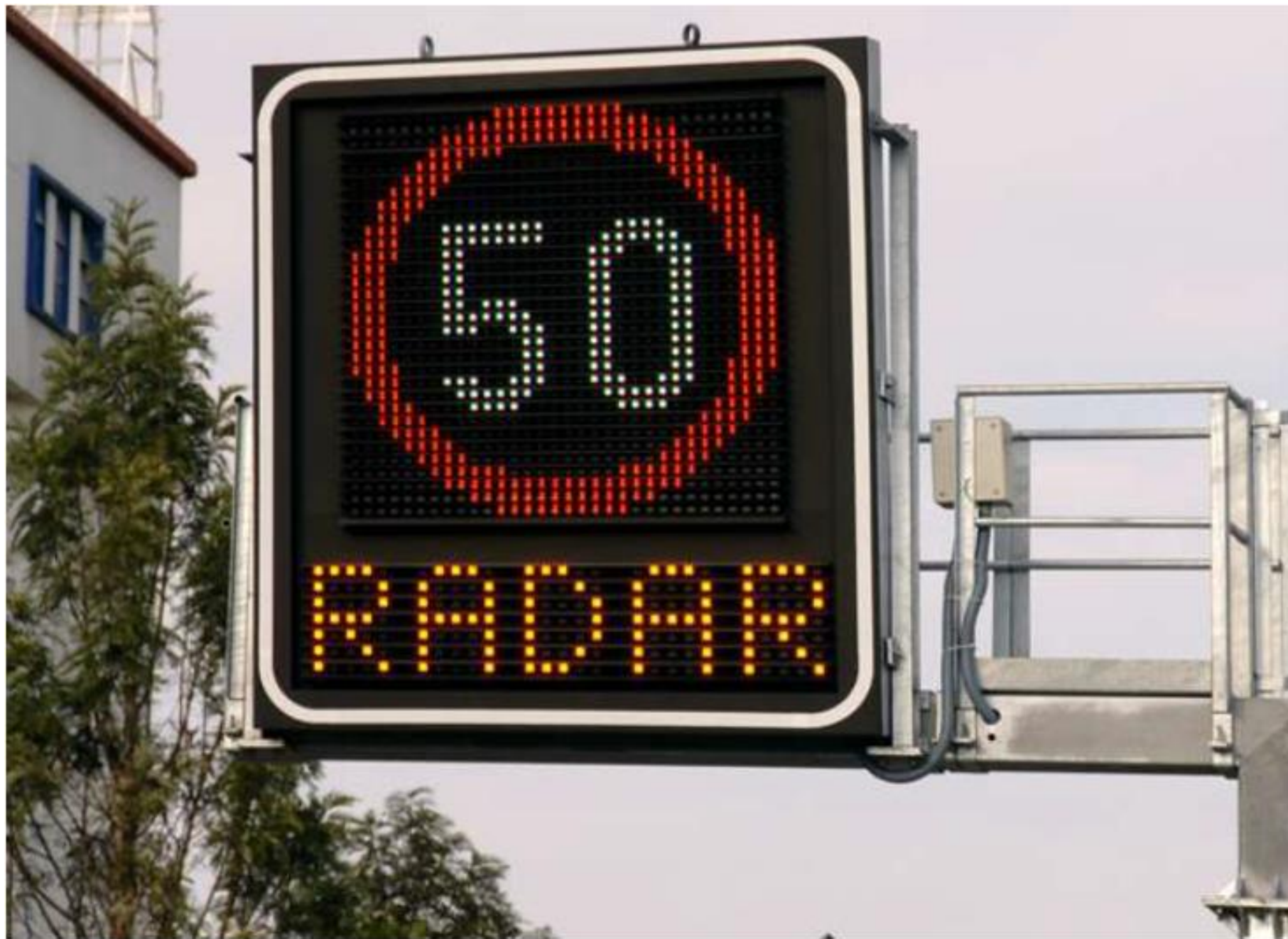
This smart road sign receives data and modifications to better inform drivers and prevent congestion or accidents.
