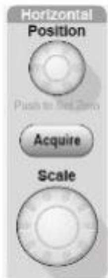
[Figure 3-15] The horizontal system controls
