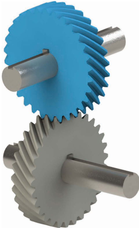
FIGURE 8.4 Mating two left-handed (or two right-handed) helical gears will transmit motion between perpendicular, non-intersecting shafts.
