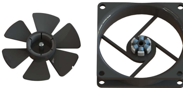
FIGURE 5.99 Brushless motors are often used for computer fans, since they generate very little electrical noise.
